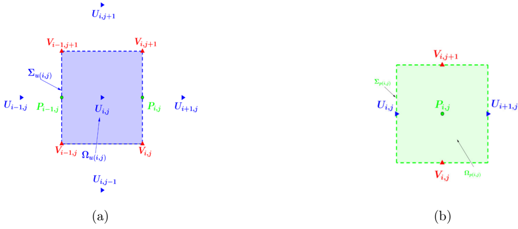
Figure 2.9: Control volume for the u velocity component, showing the locations of pressure and Eulerian velocity components (a). Control volume for pressure, showing the Eulerian velocity components (b).
